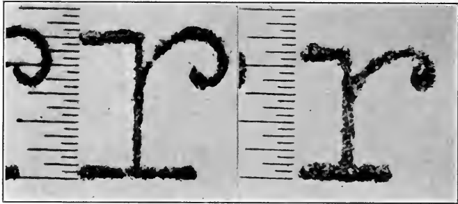
FIG. 42—Smith-Premier and Remington small r's photographed under Fig. 41 rule to show differences in size. Both enlarged thirteen and one-half diameters.
